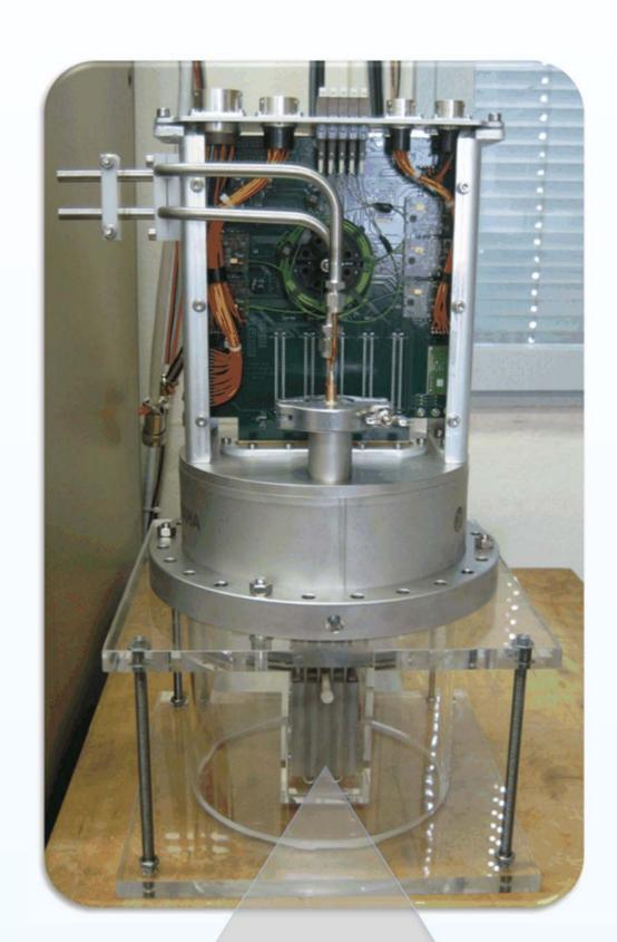
The TOTEM [1] experiment has three sub-detectors: Roman Pots (RP) with silicon edgeless microstrip silicon detector, T1 with Cathode Strip Chambers (CSC) and T2 with Gas Electron Multiplier detectors (GEM). All detectors use the VFAT [2] chip and trigger tracking tor generation mounted on different hybrids. A Roman Pot hybrid contains four VFAT chips. The set of ten hybrids is stacked and inserted in every Roman Pot.
