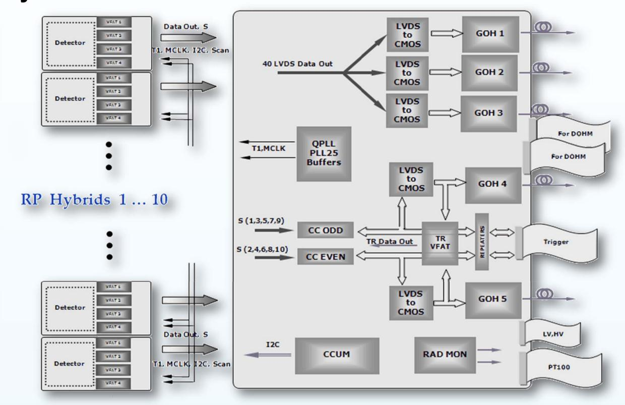
The RPMB main objectives are to acquire on-detector data and trigger from up to 10 hybrids, to perform data conversion from electrical to optical format and to transfer it to the next level of the system. It also distributes the control information to the hybrids and collects different detector and board parameters.
