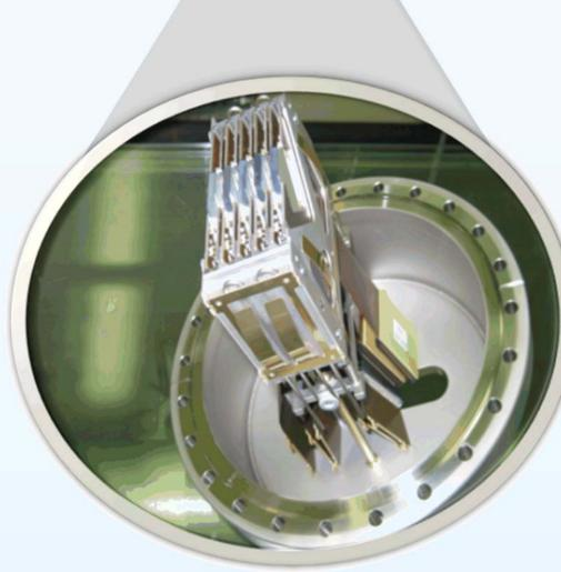
The Roman Pot Motherboard (RPMB) is connected to this set via flex connections and glued to the vacuum flange. Next is described design the and functionality of the RPMB and its components as part of the frontend electronics [3] in Roman Pot of the TOTEM experiment.
