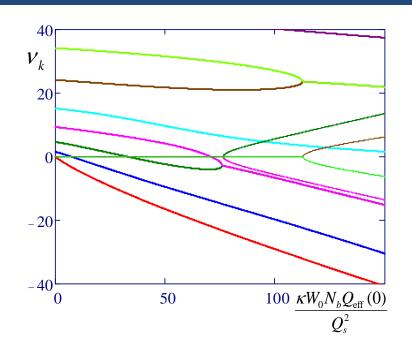
Coherent tunes of the Gaussian bunch for zero chromaticity and constant wake versus the wake amplitude.
