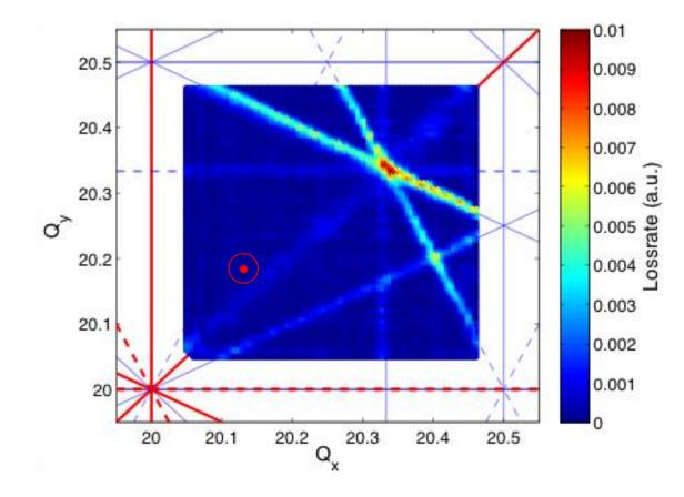
Resonance scan with low intensity single bunch beam – average of scans in all directions
