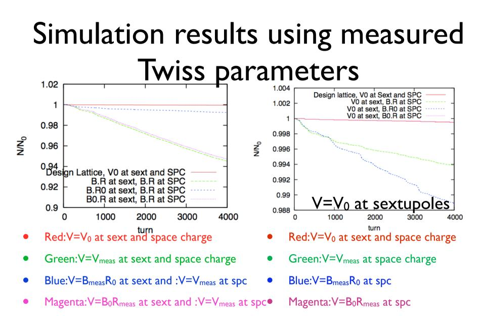
Coupling at Sextupoles is main source of the beam loss.  $\beta$  deviation does not affect in this case.
