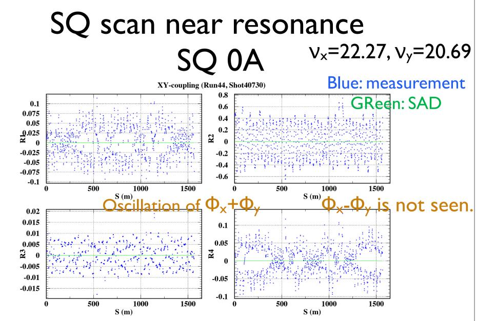
• Amplitude increases for closer  $v_x + v_y = 43$
