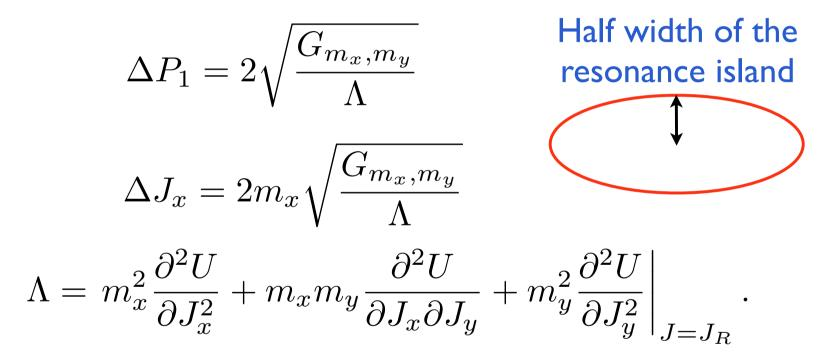
Resonance width is sqrt of the ratio of the resonance strength (G) and the tune slope (Λ)
