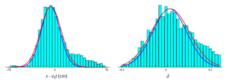
Projections onto the longitudinal coordinate (left) and  $\delta$  (right) of the original particle distribution (cyan bars) and of its Gaussian fit with  $\eta = 1$  and  $\eta = \eta_{fit}$  (red and blue solid lines respectively).
