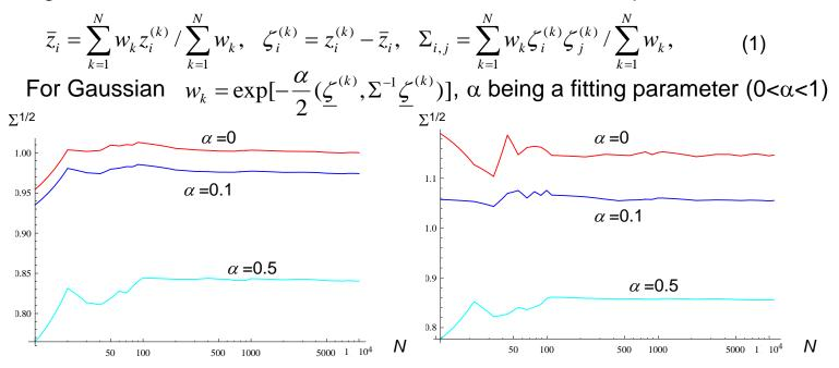
Square root of  $\Sigma$  from eq.(1) averaged over 25 realizations of 1D Gaussian distribution with  $\sigma$  =1as function of the number of particles *N*.
