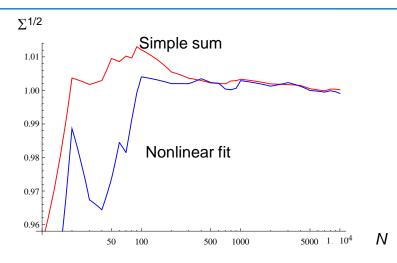
Square root of  $\Sigma$  averaged over 25 realizations of 1D Gaussian distribution with  $\sigma$  =1as function of the number of particles *N*.
