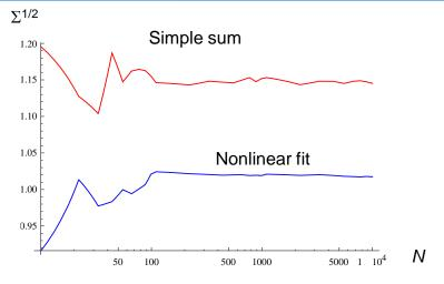
Square root of  $\Sigma$  averaged over 25 realizations of superposition of 1D Gaussian distributions with  $\sigma$  =1(90%) and  $\sigma$  =3(10%)
