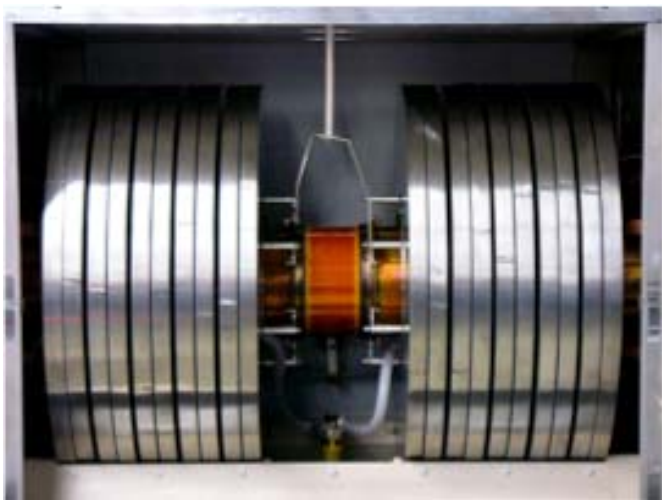
Magnetic alloy RF cavity for bunch compression
