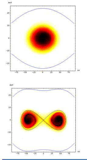
Bunch splitting at 3.5GeV/c in the CERN PS (1999/06/03). The measured data span 10ms.
