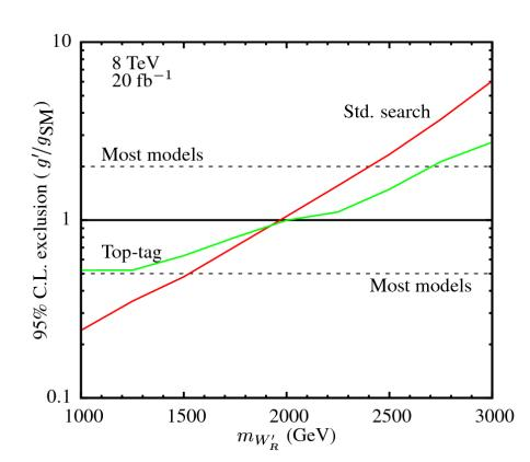
For our analysis using just a top tag on the W' > tb decay, we only reach as far as the lepton-tag method for mass, and do considerably worse at the low-mass end of the spectrum
