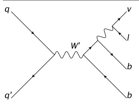
Best method of W' detection is through s-channel single top
