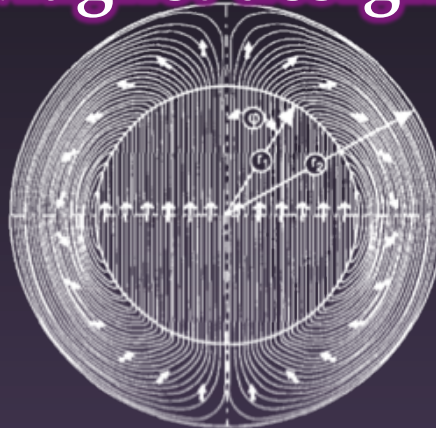
Fig. 6. Magnetic field distribution at a cross-section of the center of the magnet.
