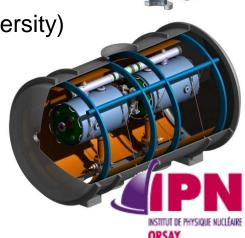
Peak fields @ 8 MV/m •  $E_{surf} = 35 \text{ MV/m}$ •  $B_{surf} = 56 \text{ mT}$ Deformation 0.25 mm Cryo loss = 15 W
