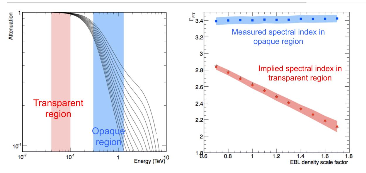
Spectral index  $\Gamma$  from fit to dN/dE ~ E<sup>- $\Gamma$ </sup> EBL model of Franceschini et al. 2008
