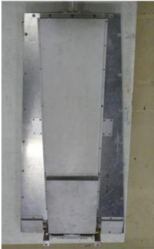
Covered by FEB shielding box
