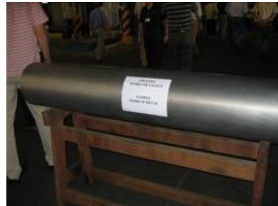
Finished RRR Nb ingot from the Pyrochlore ore
