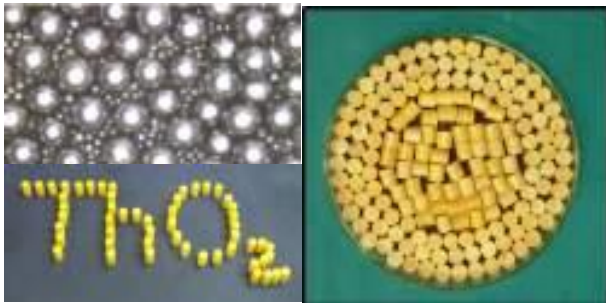
Thoria microspheres and ThO_2 Pellets fabricated for AHWR Critical Facility
