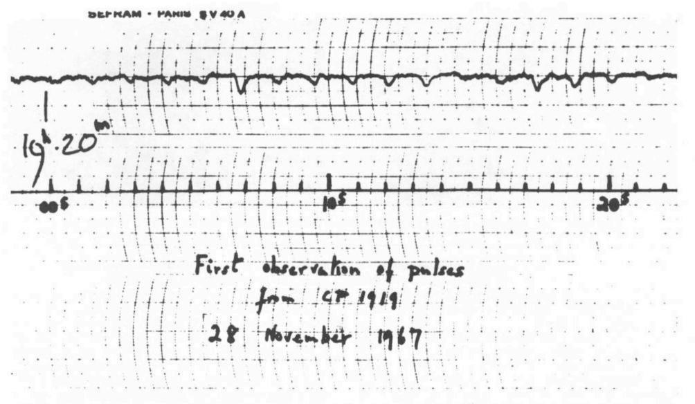
"I got it on a fast recording. As the chart flowed under the pen I could see that the signal was a series of pulses . . . 1<sup>1</sup>/<sub>3</sub> seconds apart." (Deflections are down).
