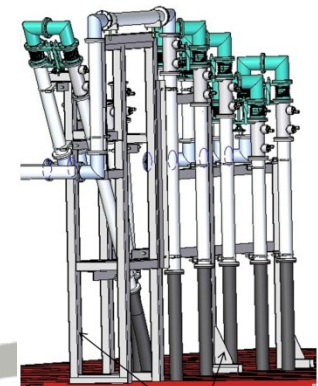
2 off Unistrut frames for coax support RFCC's - North side
