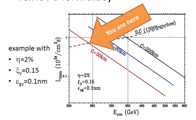
Due to a strange coincidence, the luminosity of circular and linear machines per IP at 240GeV  $E_{CM}$  are the same! (@ $\eta$ =2%)
