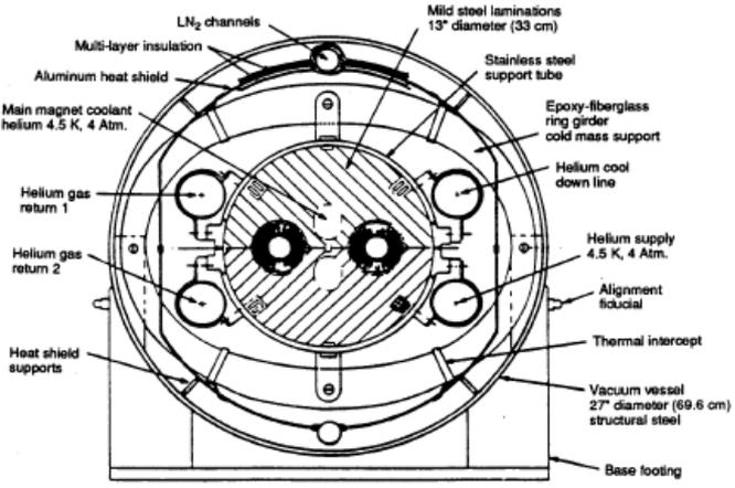
Figure 2-1. Cross section of Reference Design A dipole, including cryostat and support assembly.
