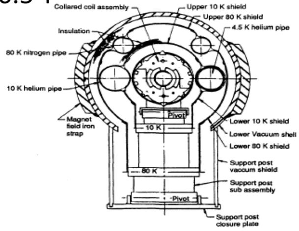
Figure 2-3. Reference Design B dipole and cryostat cross section.
