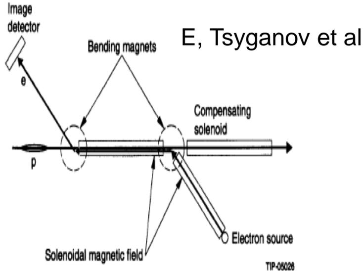
Figure 5. Schematics of a beam-beam compensating device. A low-energy electron source collides with a bunch of protons. Electrons are kept stable in space by a solenoidal magnetic field. After collision with the proton bunch, an electron beam is deflected to the image detector, which is used to steer the electron beam relative to the proton bunch.
