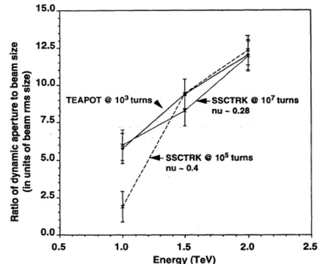
Figure 8-1. Graph of Calculated Dynamic Aperture versus Injection Energy.
