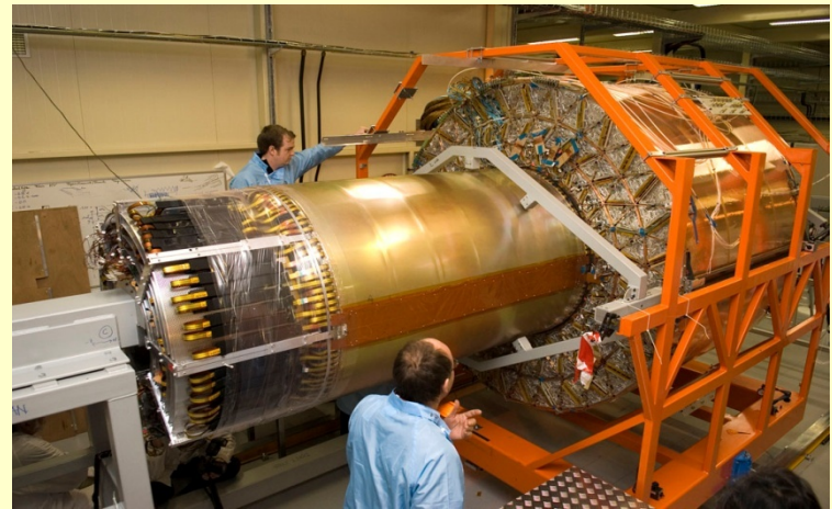
SCT-TRT integration in the surface building.(Feb. 2006)
