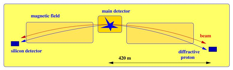
Forward Proton measurement – 420 meters downstream
