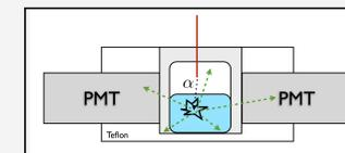
Two pmts face a sample of QDs or scintillator.
