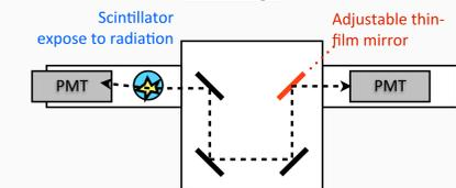
Built spectrometer to measure emission spectra of scintillation light
