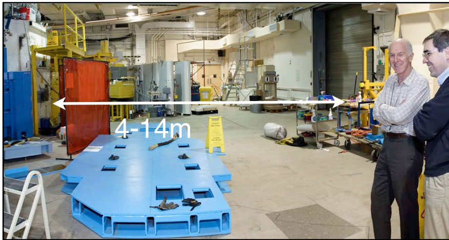
Possible detector baselines at NIST 3.8m, 6.8m, 11.8, 15.2m (up to 20m)
