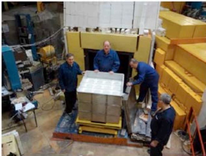
Installation of 2 sections test antineutrino detector with liquid scintillator (total volume 0.4 m 3 )
