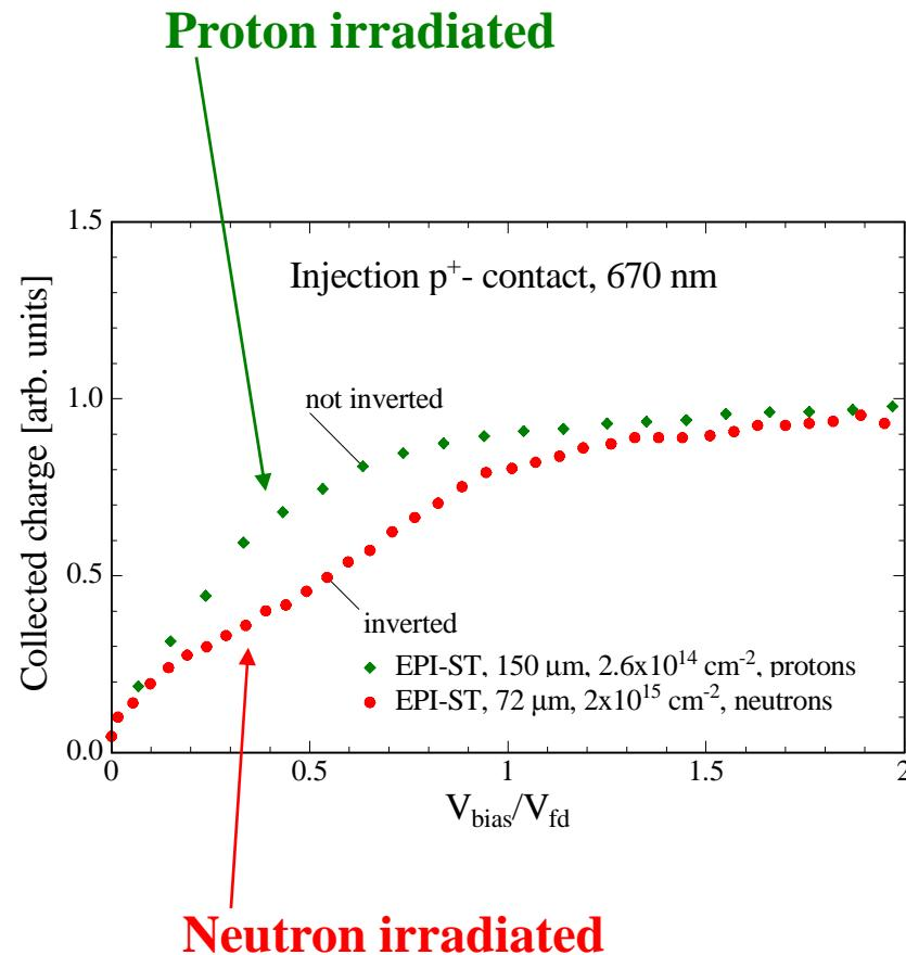
Illumination of p+-contact with 670 nm laser light (absorption length at RT about 3 μm):
