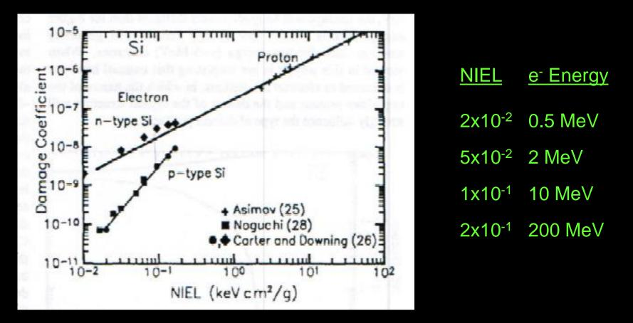
Damage coefficients less for p-type for  $E_{e^-} < ~1$ GeV (two groups); note **critical energy** in W is ~**10** MeV **But**: Are electrons the entire picture?
