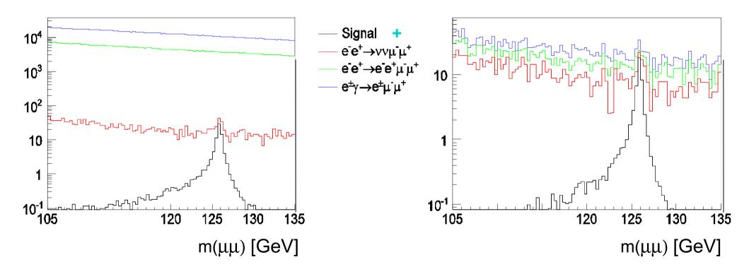
Reduction of the dominant  $e^+e^- \rightarrow e^+e^-\mu^+\mu^-$  background by factor 1000 Background with the identical  $\mu\mu\nu\nu$  signature can't be further suppressed
