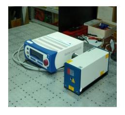
The first step: the tunable laser was purchased to laboratory power 10mW wavelength range: 663 – 678 nm
