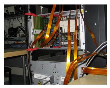
LAB - system prototype with optical movable table 2D Studies on the behaviour of the sensors, laser beam and calculation of the prototype displacements in ref. frame - actual accuracy.
