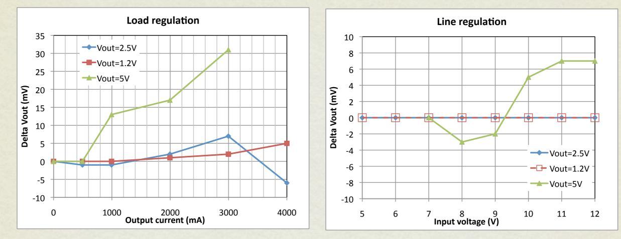
Conditions: cooling plate at about 18C, L=430nH oval toroidal (bulk Cu wire), f=1.8MHz
