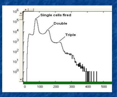
There are other ways fake pulses to be produced – crosstalk and after-pulsing. They can be induced by both dark pulses and incoming light pulses
