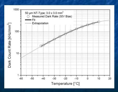
Significant disadvantage of the SiPM is the presence of dark pulses.
