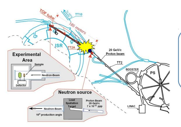
n\_TOF is a spallation neutron source based on 20 GeV/c protons from the CERN PS hitting a Pb block (~350 neutrons per proton).
