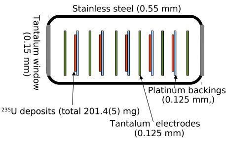
The PTB chamber is calibrated, meaning that the mass of <sup>235</sup>U and the detection efficiency are well known from previous "international intercomparisons".
