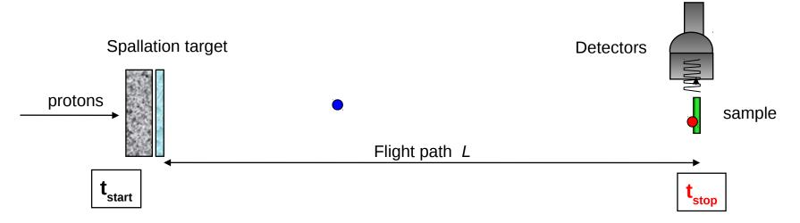
The accurate determination of **neutron cross sections** requires a high accuracy knowledge of the **neutron flux** (typically within 1-3 %)
