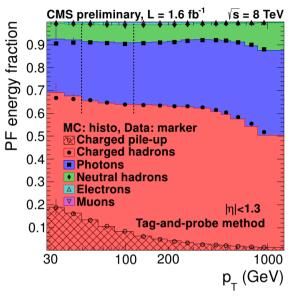
CMS has need for very detailed understanding of fraction of different particles per jet and fraction of pile-up particles in jet as these are subtracted by the particle flow algorithm
