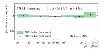
Efficiency measured in top and QCD events (data) using multiple methods
