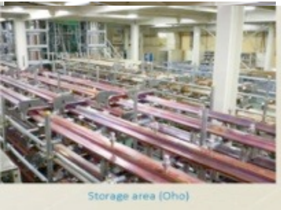
Beam pipes after baking and TiN coating in a stock area.
