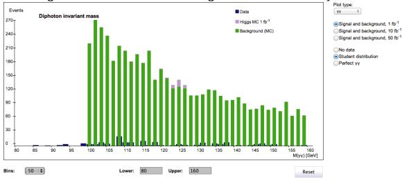
To claim discovery, ATLAS analysed more than 10fb<sup>-1</sup> of data. The next figure demonstrates that with 50fb<sup>-1</sup>, for example, a clear signal singles out on top of a smooth exponential background.
