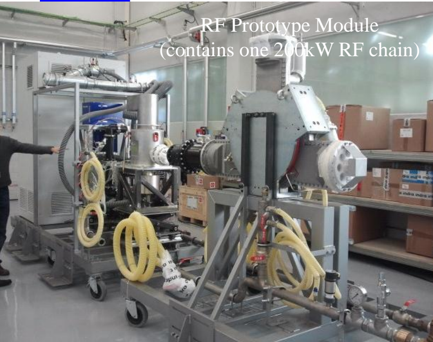
One Module contains two RF Chains
