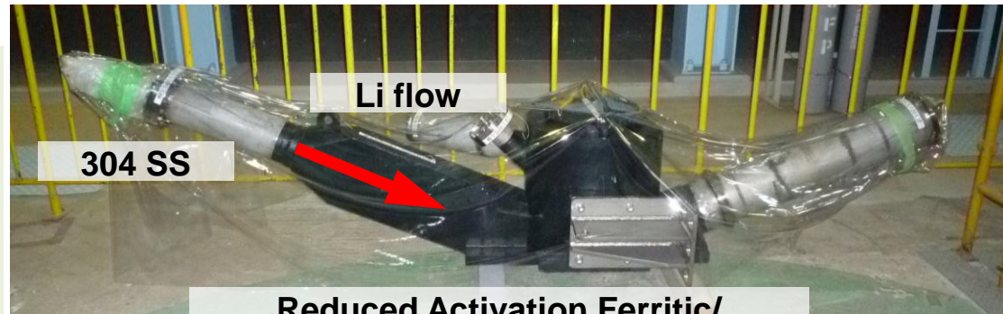
Reduced Activation Ferritic/ Martensitic Steel, F82H, target body
