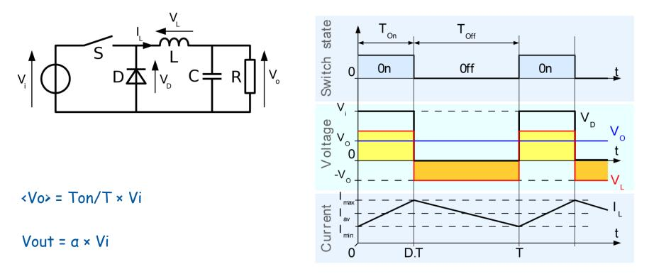
The output voltage can be controlled by playing with the duty cycle a.
