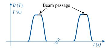
Direct Energy transfer from mains is not possible: Intermediate storage of energy Peak power : could be > MW Average power kW
