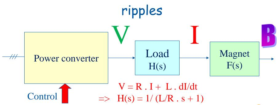
Voltage ripple is defined by the power supply
