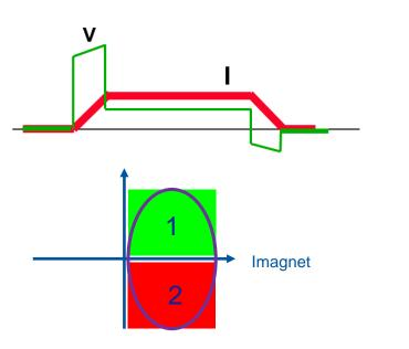
12 converters in series between magnets. Each converter gives 6kA/2kV.
