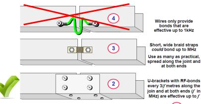
But continuously seam-welded or conductively-gasketed joints are best (1
