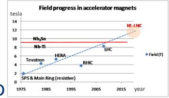
performance of Nb<sub>3</sub>Sn wires has seen a great boost in the past decade (factor 3 in J<sub>C</sub> w/r to ITER)
