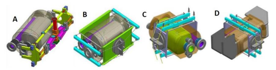
Figure 1: LHC crab cavity cryostat concept – A) JLab design, B) ANL design (helium pressure actuates bellows), C) ANL design (tuner deforms cavity outer surfaces), D) Waveguide
