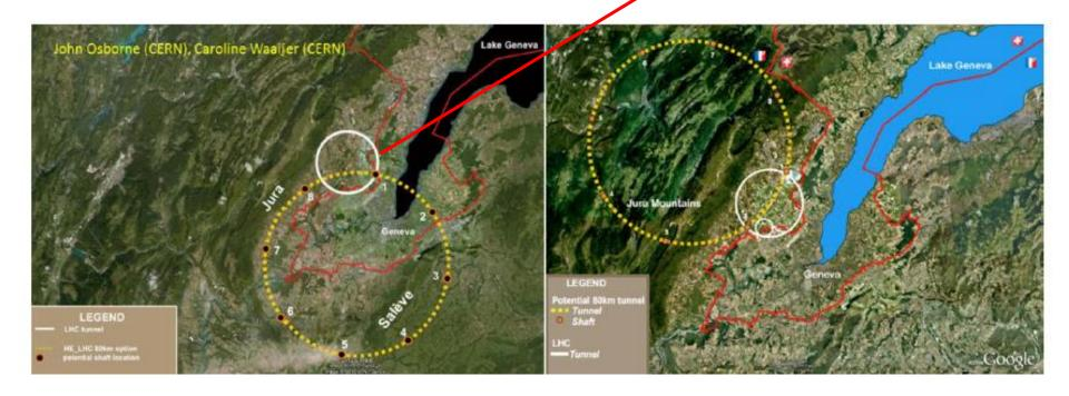
80-100 km tunnel infrastructure in Geneva area – design driven by pp-collider requirements with possibility of e+-e- (TLEP) and p-e (VLHeC)
