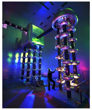
750 kV Cockroft-Walton generator at Fermilab (Proton source)
