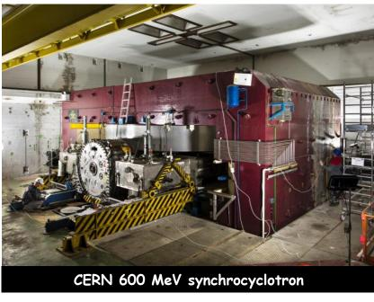
Synchrocyclotron: Same as cyclotron, except a modulation of  $\omega_{\mathsf{RF}}$
