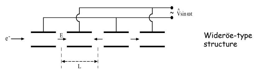
Cylindrical electrodes (drift tubes) separated by gaps and fed by a RF generator, as shown above, lead to an alternating electric field polarity
