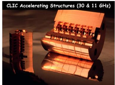
solution: slow wave guide with irises ==> iris loaded structure
