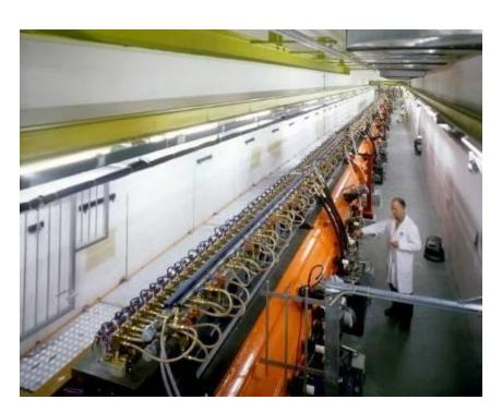
Top; CERN Linac2 Drift Tube Linac: 1978, 202.5 MHz, 3 tanks, final energy 50 MeV, tank diameter 1 meter.
