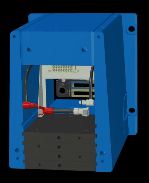
➤ Bypass the fLVPS cooling hoses by connecting them to each end of the bypass cooling hose
