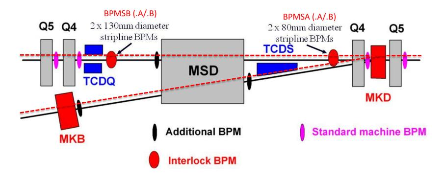
The main aim of these BPMs is to avoid large orbit offsets leading to high losses on the septum protection during a dump
