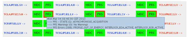
Figure 4: Collimator status display with detailed error and warning messages.
