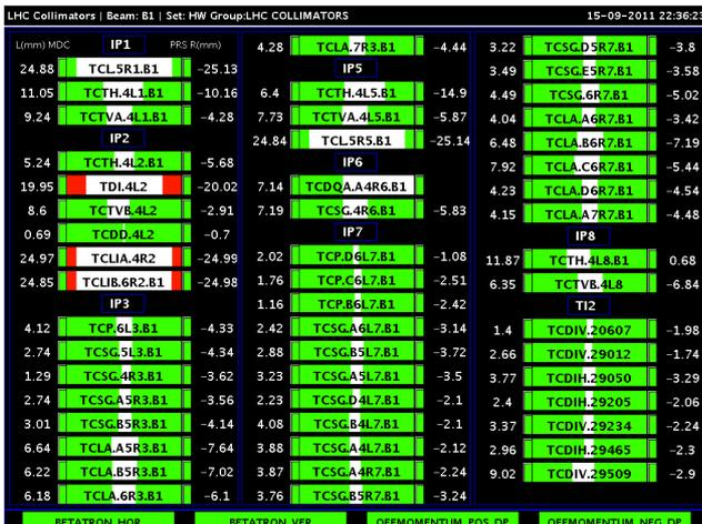
Figure 3: Collimator statuses and jaw positions B1 visistar [9].
