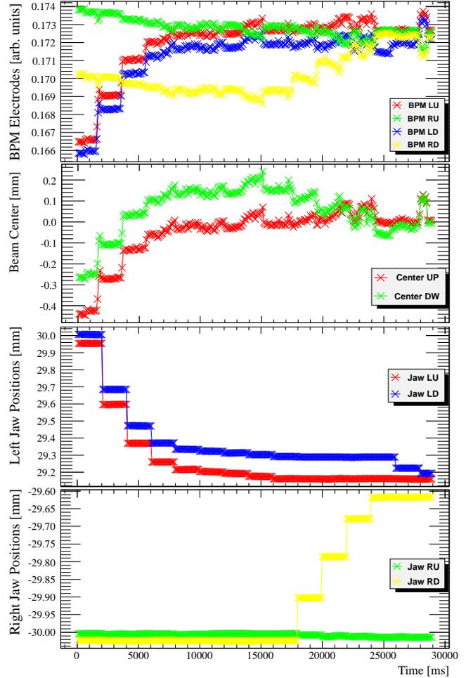
Figure 8: BPM-based collimator alignment [15].
