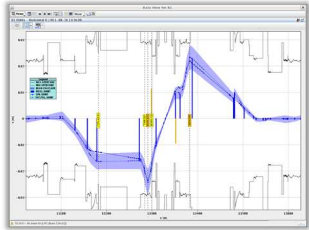
Figure 10: Example live plot of the LHC Aperture Meter. It shows the beam in an IP, together with an envelope of 1\sigma and the aperture limits.
