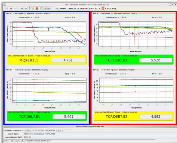
Figure 9: Main Screen of the LHC Aperture Meter. For each beam and plane it shows the distances of the five elements closest to the beam over time.
