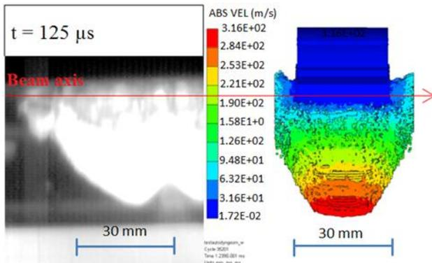
Figure 11: Comparison between simulation (SPH method) and acquired image  $\sim 125 \mu s$  after the impact.
