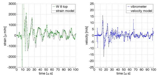
Figure 9: Comparison at  $r = 20 \text{ mm}$ ,  $L = 15 \text{ mm}$ , measurements (dotted lines) vs. simulations (continuous lines); axial strain (left) and radial velocity (right).
