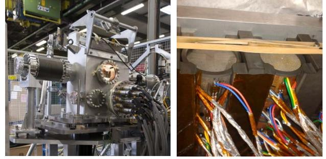
Figure 8: Assembled test-bench with DAQ cables and connectors (left); strain gauges mounted on Molybdenum-Copper-Diamond and Copper-Diamond (right).
