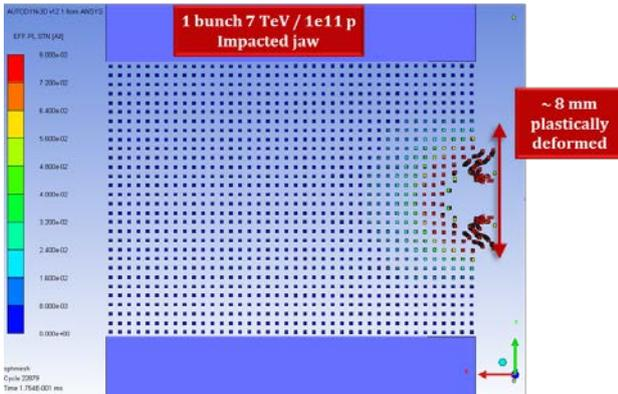
Figure 14: Threshold 3,  $1 \times 10^{11} p$ : groove generated in the jaw; Below this threshold the damage can still be compensated through 5<sup>th</sup> axis movement.
