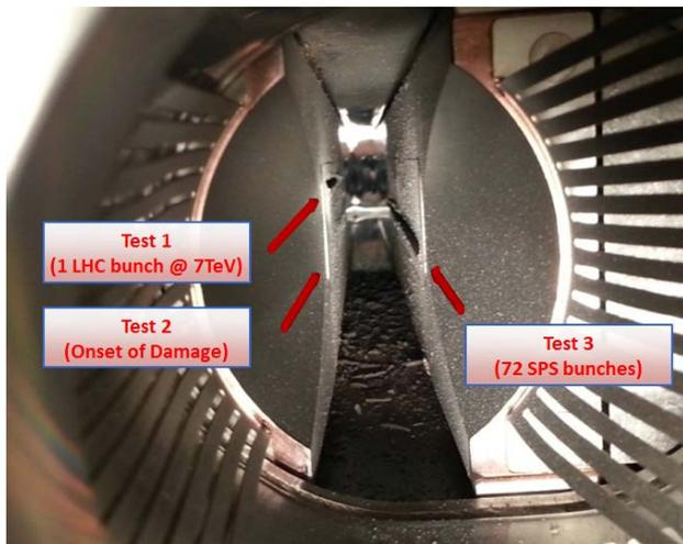
Figure 2: Post-irradiation visual inspection. Note the impressive quantity of tungsten ejected (partly bonded to the opposite jaw, partly fallen on tank bottom or towards entrance and exit flanges).
