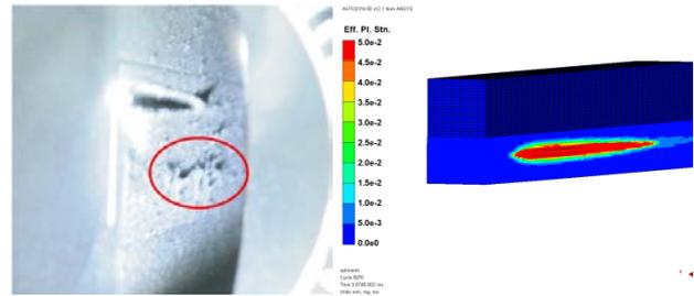
Figure 4: Qualitative numerical benchmarking of the damage generated by Test 2 beam impact. Note that the impacted zone is covered by particles ejected from the opposite jaw during Test 3.
