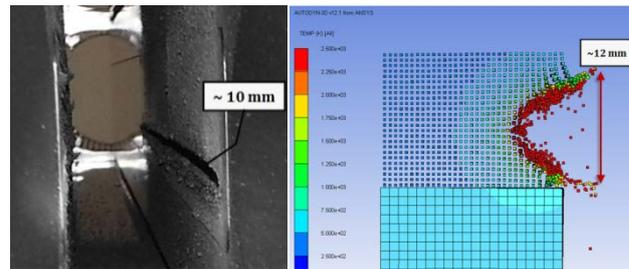
Figure 5: Qualitative numerical benchmarking of the damage generated by Test 3 beam impact.
