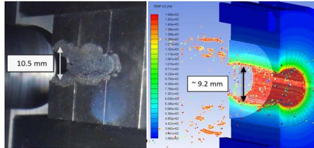
Figure 12: Post-mortem observation of Inermet® 180 samples (left) and simulated failure (right).
