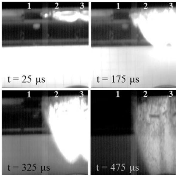
Figure 10: Image sequence of the impact on Inermet® 180 at high energy; three samples are partially visible.
