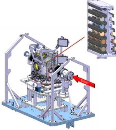
Figure 6: General assembly of the HRMT-14 test-bench.
