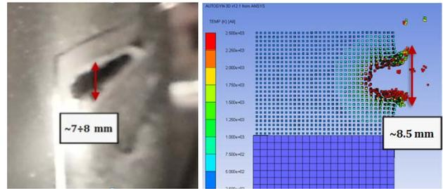
Figure 3: Qualitative numerical benchmarking of the damage generated by Test 1 beam impact.
