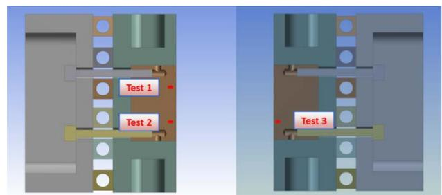
Figure 1: Schematic diagram of the three tests performed on the TCT during HRMT09 experiment. Impact locations are shown in red.
