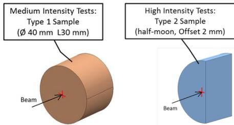
Figure 7: Material specimen shapes for medium intensity (type 1 - left) and high intensity (type 2 - right).
