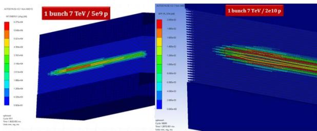
Figure 13: Threshold 1,  $5 \times 10^9 p$ : no plastic deformation induced (left); Threshold 2,  $2 \times 10^{10} p$ : a crack is generated, but without ejection of tungsten particles.
