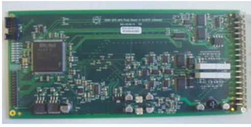
Figure 1: Radiation tolerant, FPGA based quench detection board type DQQDI used for the protection of insertion region magnets.
