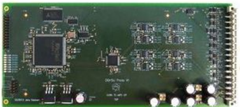
Figure 2: Dedicated DAQ board type DQHSU for the supervision of quench heater circuits.
