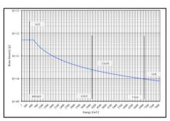
After LS1 the LHC will be operated at an energy close to 7 TeV. The value of the normal setup beam flag would in this case allow an intensity of ~1x10<sup>10</sup> (pilot beam)
