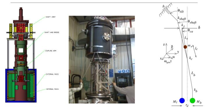
GG in space needs no motor no bearings, has no "terrain" tilts, has weaker coupling and higher sensitivity by 3 orders of magnitude; the driving signal from Earth is 500 times stronger ...yet the key features are the same as in GGG
