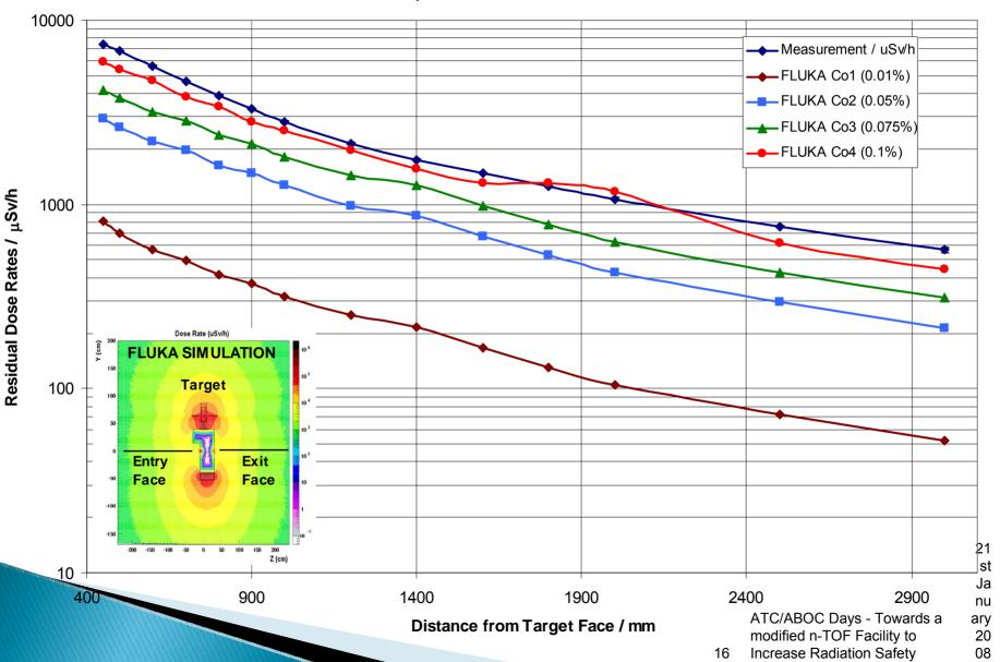
Residual Dose Rate Scan - Entry Face New FLUKA Comparison for Different Cobalt Contents
