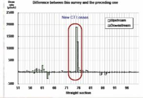
PS bridge problem cured by displacing beam losses from section 5 to 73
