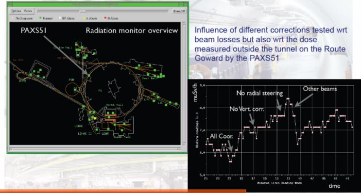
Radiation is caused by losses during injection – difficult to minimize more
