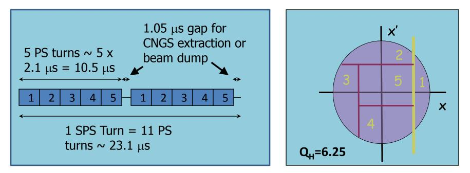
Inherent losses of around 10-12% due to the thickness of the septum and the large trajectory excursions around the machine.
