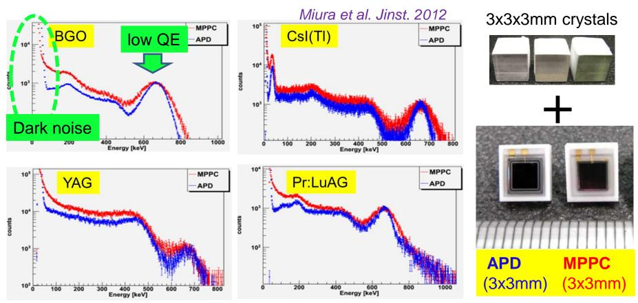
Measurements w/ APD/MPPC couple w/ small cubic scintillaotrs irradiated by 662 keV gamma-rays
