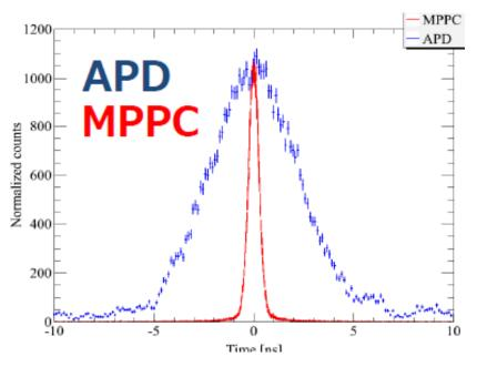
Back-to-back measurements of 511 keV gamma-rays
