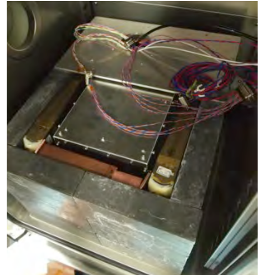
lead shield (5cm thick)、copper/brass shield (1cm-5cm thick)、aluminum case( several mm thick)
