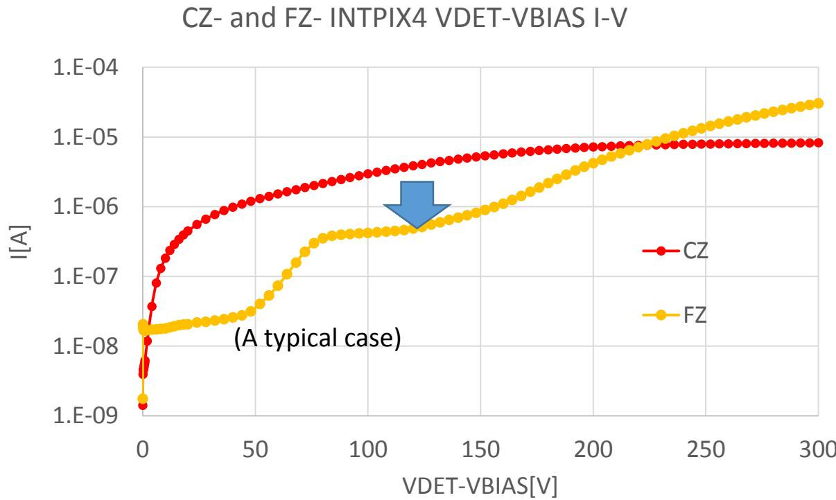
Leakage current is lower in FZ SOI sensors.
