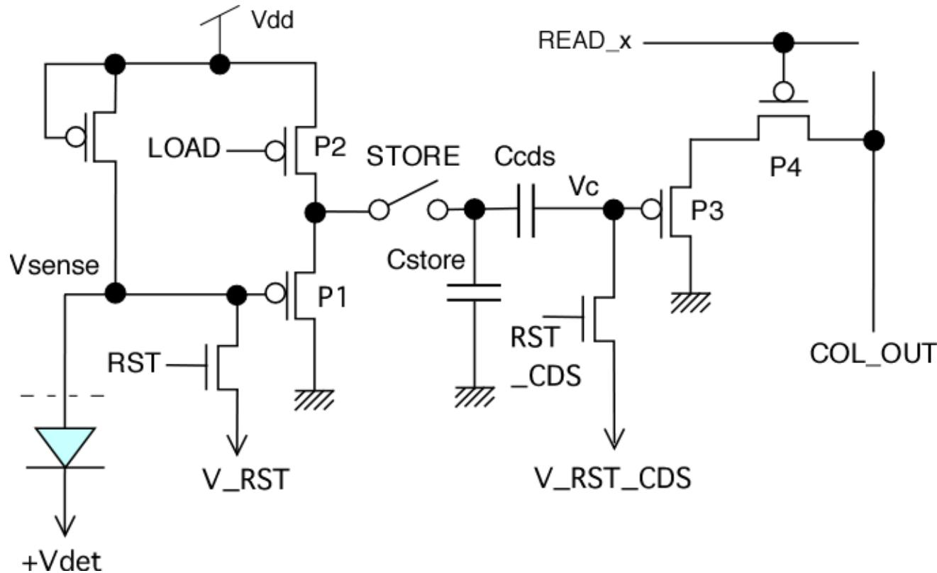
The pixel circuit has CDS function.
